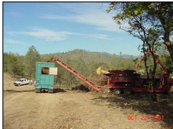
Biomass Collection in Action. Tub grinder on right, conveyor moves biomass into the
