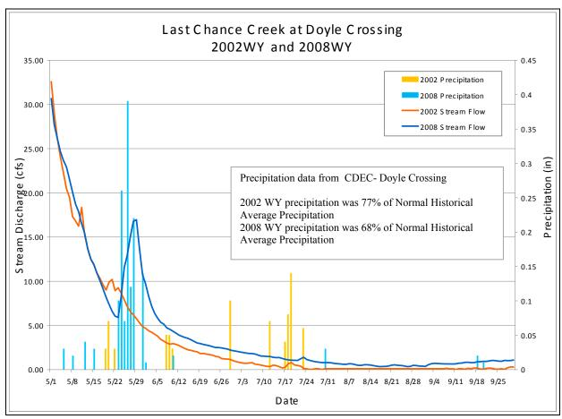
Figure 12: Spring recession stream flows in 2002WY and 2008WY at Doyle Crossing
