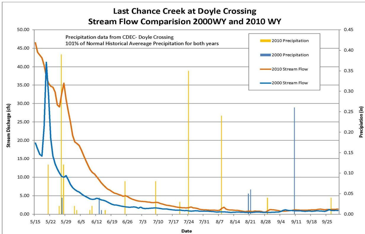
**Figure ES-2:** Last Chance Creek summer stream flow measurements for near-normal water years at Doyle Crossing, 2000 and 2010. Approximately 9 miles of pond-and-plug restoration was implemented upstream of this gage from 2003 through 2007 (see Figure ES-3). There is no statistical trend in late season flow amounts at Doyle Crossing.
