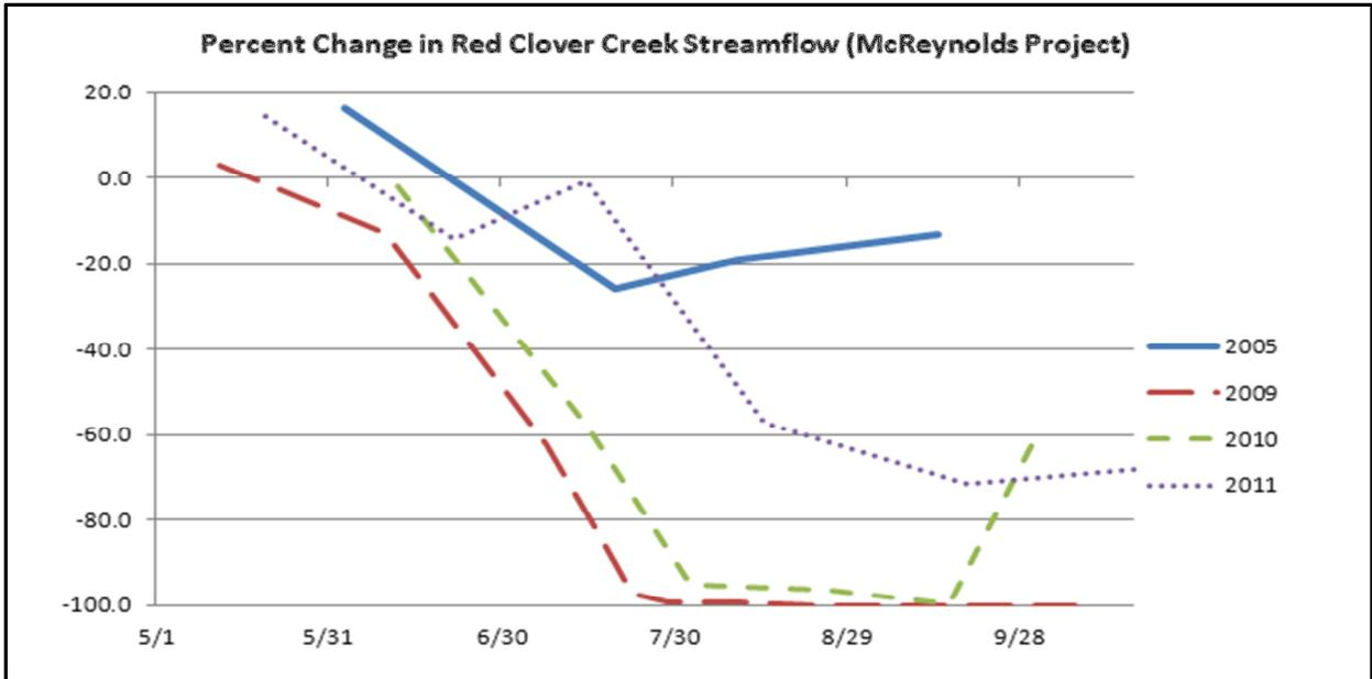
**Figure ES-1:** Percent change in streamflow occurring between top and bottom of McReynolds project. 2005 is pre-project. For the post-project period (2009 – 2011), rates of surface flow loss are substantially higher. 2005 and 2010 had near-normal annual precipitation. 2009 was below normal. 2011 was above normal.
