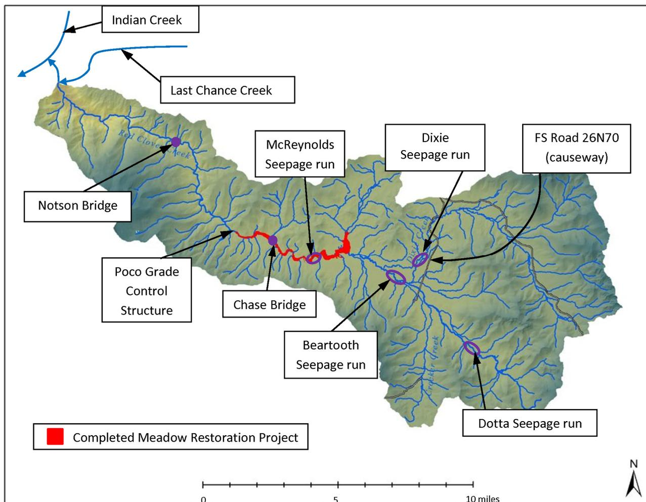
**Figure 9** - Stream flow measurement and Seepage Run locations in the Red Clover Creek watershed
