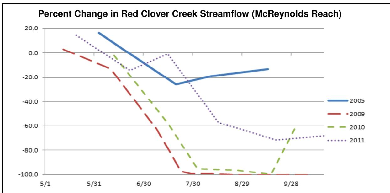
**Figure 6-** Percent change in streamflow occurring between top and bottom of McReynolds project. 2005 is pre-project. For the post-project period (2009 – 2011), rates of surface flow loss are substantially higher. 2005 and 2010 had near-normal annual precipitation. 2009 was below normal. 2011 was above normal.
