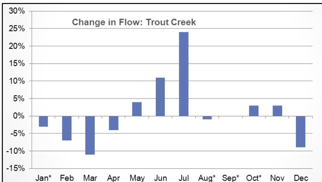
**Figure 2-** Monthly changes in flow from Trout Creek (from Tague, et al). Asterisks are added for January, August, September, and October because the observed changes between pre- and post-project flows were not statistically different.
