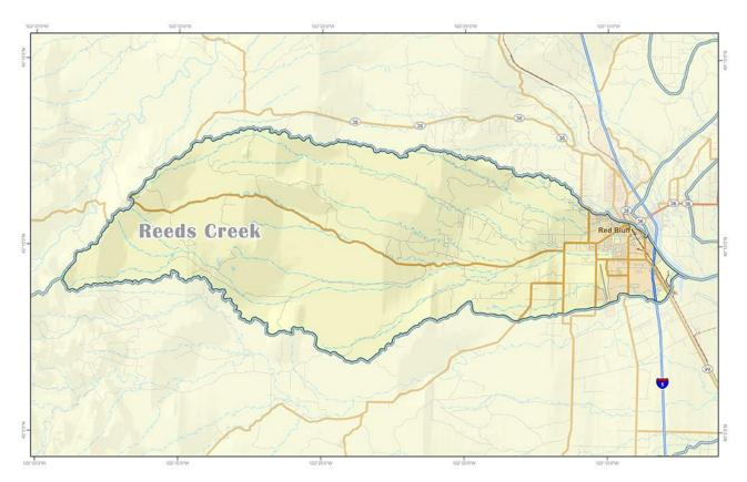
Reeds Creek flows 22 linear miles from an elevation of 1,100 feet to the Sacramento River at the 253-foot elevation level. Principle tributaries to this significant westside stream are Brickyard, Pine, Liza, and Live Oak Creeks. The watershed of Grasshopper Creek near the Sacramento River is also included. Blue oak woodlands, grasslands, live oak/riparian woodlands, and cultivated lands occupy most of the planning unit. The Red Bluff urban area occupies about 4% of the total watershed area.
