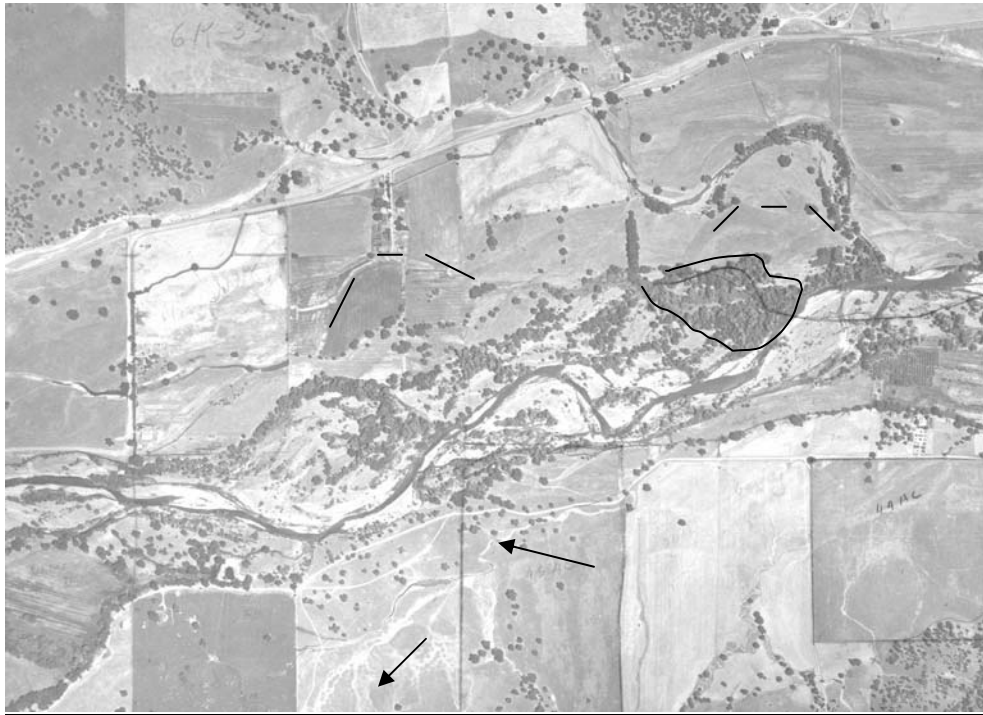
Figure 8a (top, 1952) and 8b (bottom, 2004). Significant areas of riparian growth that have been affected are circled by black lines. Gully erosion features are shown with arrows. Note old stream bend features shown with broken lines. This is Site 5.
