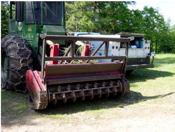
**Figure 9.** Vertical Shaft Masticator with wheels.
