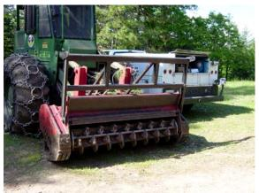
Figure 9. Vertical Shaft Masticator with wheels.
