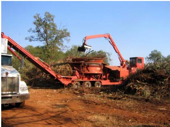
**Figure 13.** A Morbark tub grinder processing debris.
