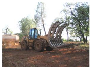
Figure 12. A Caterpillar 996 loader moves woody debris to grinder.
