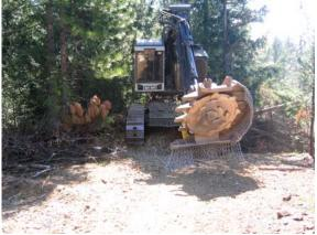
Figure 10. Horizontal Shaft Masticator with treads.
