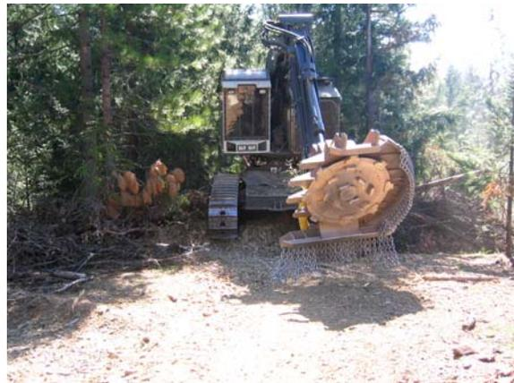
**Figure 10.** Horizontal Shaft Masticator with treads.
