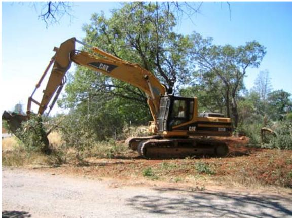
**Figure 11.** A Caterpillar 325 excavator with thumb.
