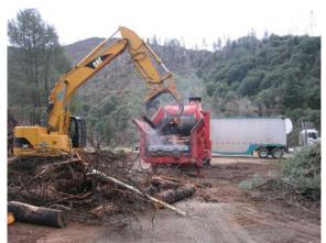
Figure 7. Loader placing material into chipper.
