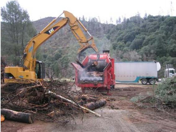
**Figure 7.** Loader placing material into chipper.
