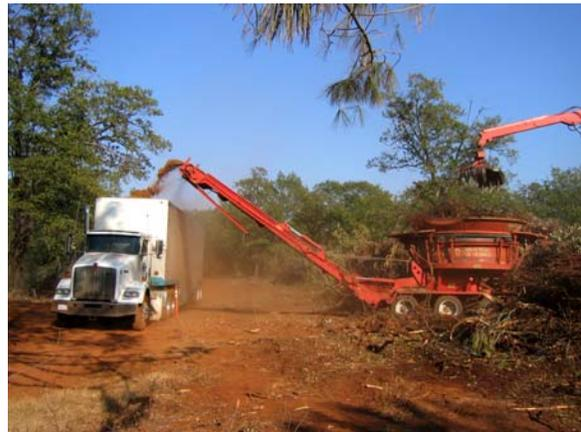
**Figure 14.** A chip van being loaded.
