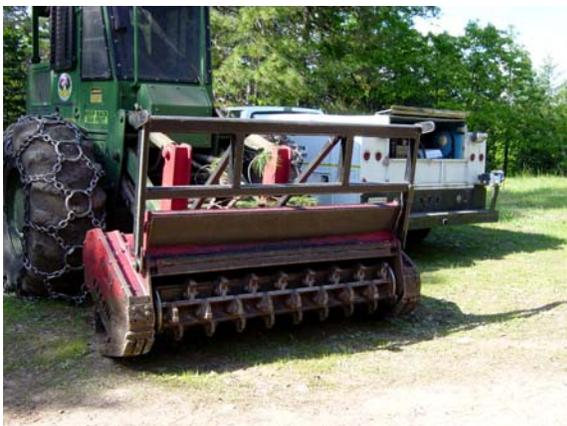
**Figure 9.** Vertical Shaft Masticator with wheels.
