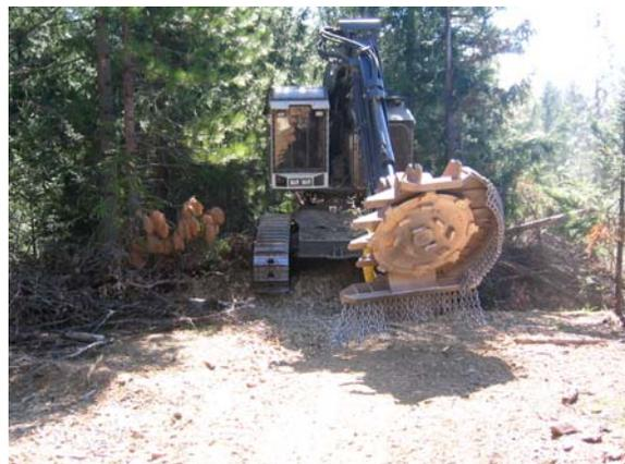
**Figure 10.** Horizontal Shaft Masticator with treads.
