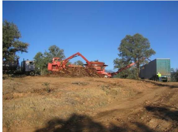
**Figure 8.** Chip van being loaded.
